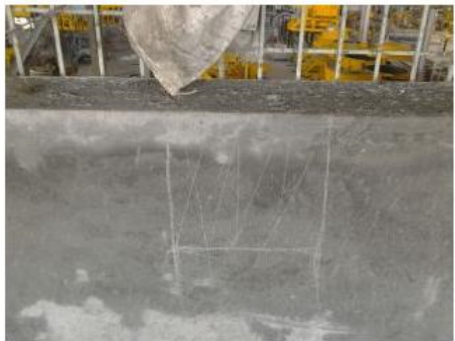
During the Scratch test on plaster
