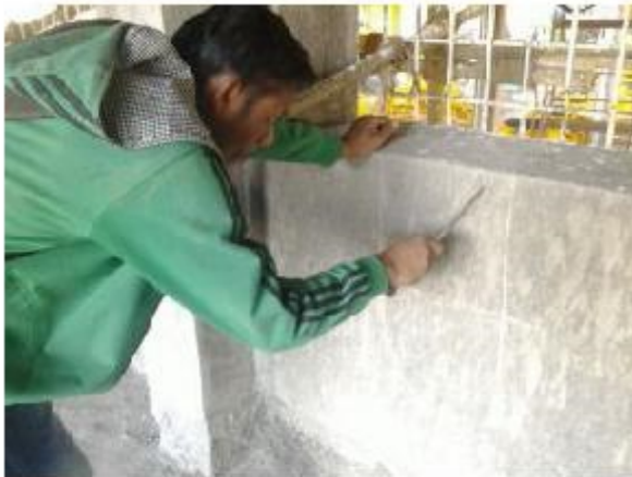
During the Scratch test on plaster
