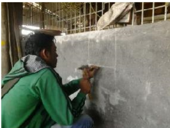
During the Scratch test on plaster
