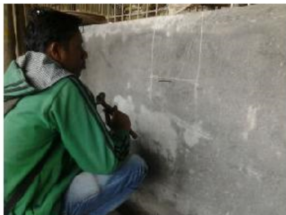
During the Scratch test on plaster
